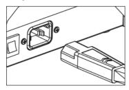
• Attach the nut at the end of the air hose to the air outlet on the turbine ensuring it is screwed on fully. The connection will be rigid when fitted correctly.
