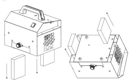
Check the condition of filter carefully and replace if necessary.
